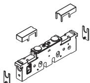
intermediate supply plate with open exhausts and external pilot supply weight: 0,164 Kg
