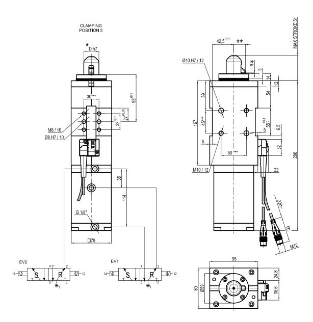
\*\* MISSING DIMENSION TO BE DEFINED ACCORDING TO CUSTOMER SPECIFICATIONS \*\*\* TOLERANCE BETWEEN DOWEL HOLES  $\pm$  0,02, BETWEEN SCREW HOLES  $\pm$  0,1
